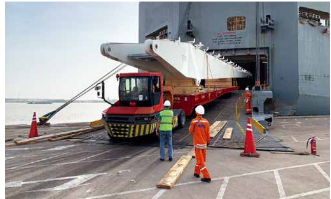
Loading scene of a crane jib
